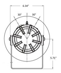
\* All versions are fitted with one (1) 1/2 inch NPT entry and two (2) 20mm entries. The 20mm entries are fitted with brass stopping plugs as standard. In addition a ½" NPT brass stopping plug is provided.
